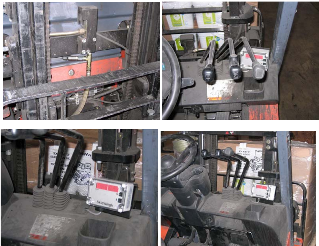
Example of the pressure transducer installation / digital indicator on Toyota forklifts with short mast
