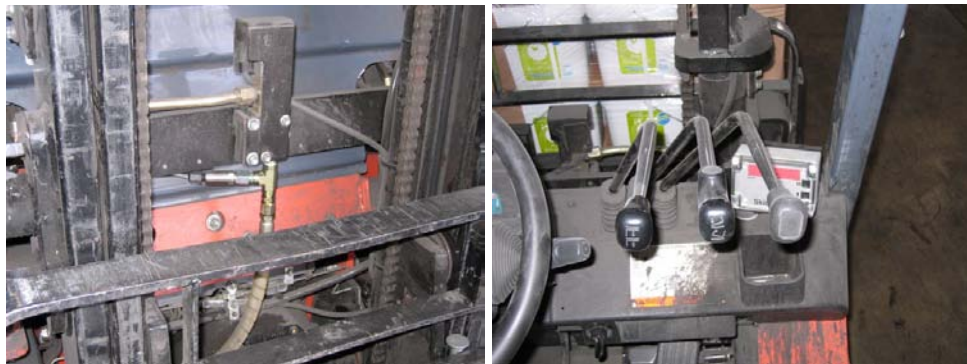
Example of the pressure transducer installation / digital indicator on Toyota forklifts with short mast
