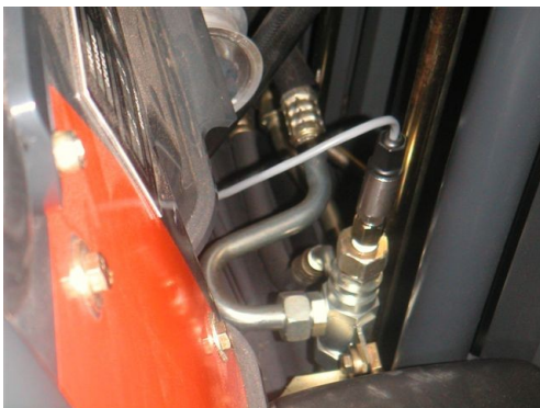
Typical Hydraulic Pressure Transducer Installation
