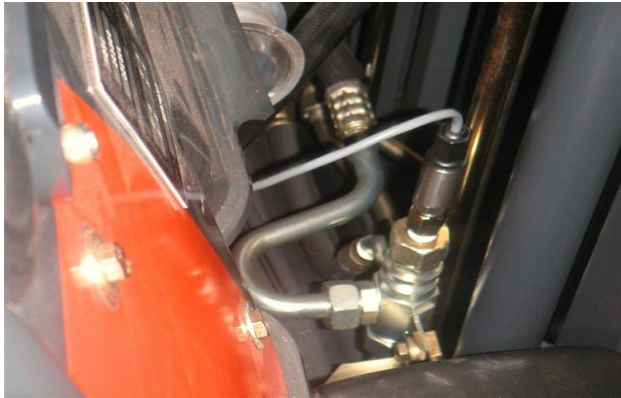
Typical Installation of the ED2 Series Pressure Transducer in Lifting Hydraulic Circuit
